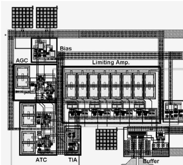
Fig 9. Layout of the burst-mode front-end circuit
