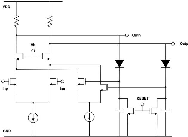
Fig 6. Limiting amplifier with offset cancellation
