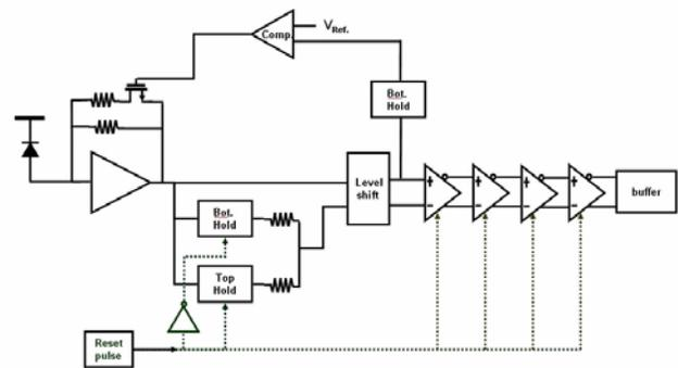
Fig 2. Block diagram of the burst-mode optical receiver
