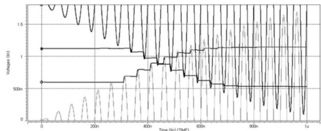
Fig 5. Top and bottom hold circuit detection range
