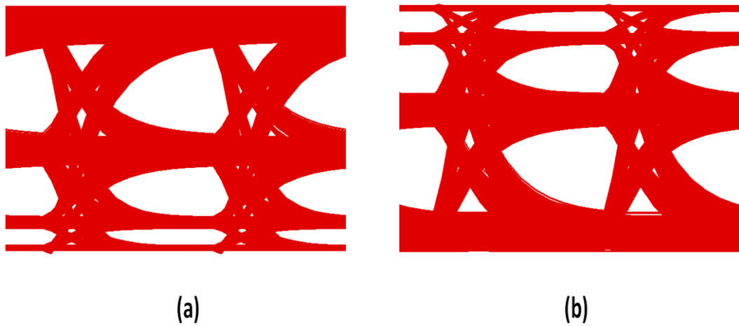
Fig. 4-25. PAM-4 50 Gb/s simulation results for behavior of RLM control buffer with (a) downside clipping, (b) upside clipping
